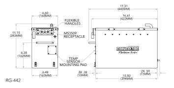
Concorde's superior Platinum Series® batteries have been proven reliable, durable and safe in turbine aircraft applications for more than two decades. Concorde's valve regulated sealed recombinant gas (RG®) Turbine Starting aircraft batteries are constructed with advanced lead acid, absorbed glass mat (AGM) technology.
